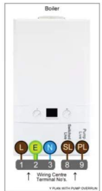
Y Plan with Pump Overrun
